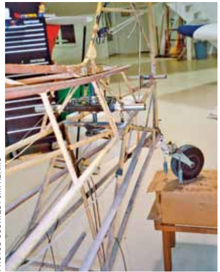
The aft section of the fuselage, after the old fabric was removed—note the wood stringers.
