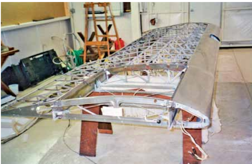
The wing, with the original truss-style ribs.
