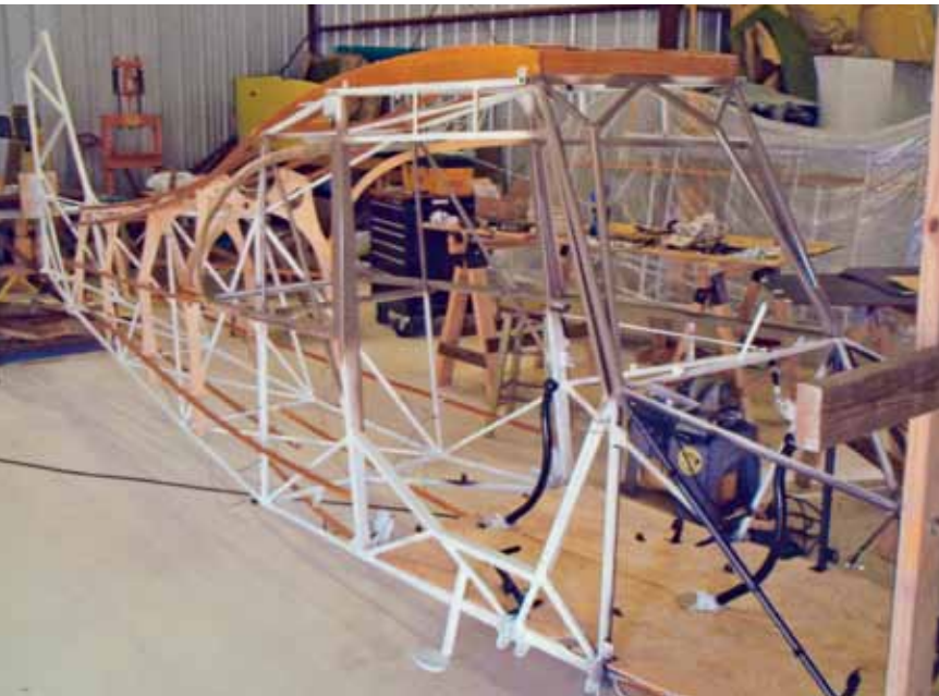
The refurbished fuselage, replete with stringers and formers.
