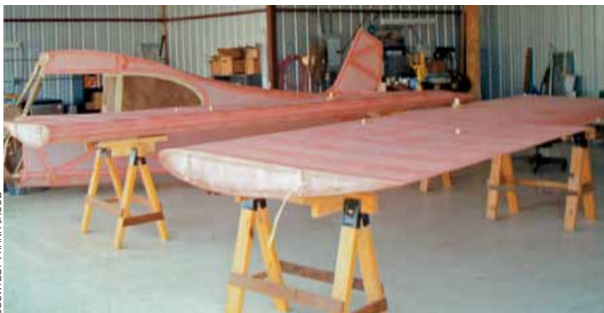
The fabric-covered fuselage and wings, coated with Poly-Brush.
