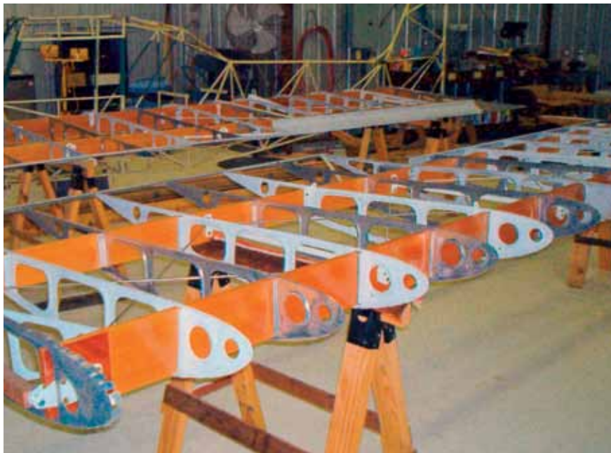
New and old ribs are mounted on the new spruce spars.
