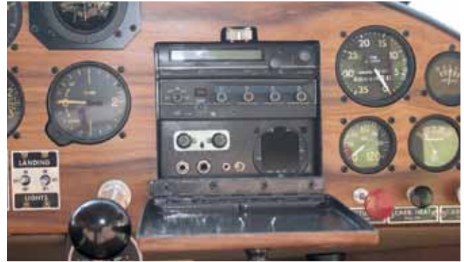
The original glove box neatly conceals a modern transponder, radio, and engine analyzer.
