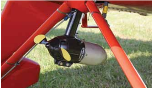
Serial number 828 came from the factory with a wind generator.
