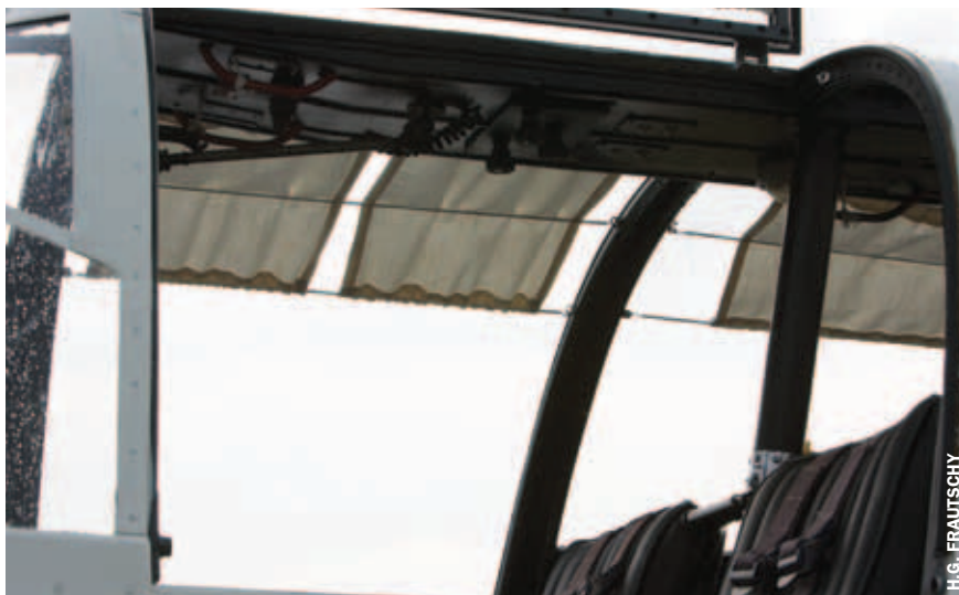
The cowling for the 180-hp Lycoming has its outlets for the cooling air on the side. The amount of deflection for the side vents can be adjusted on the ground.
