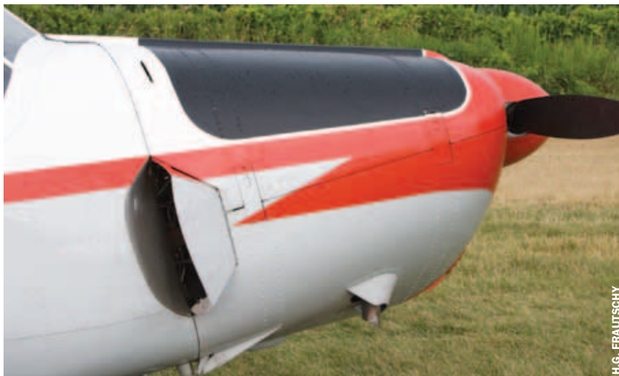
The cowling for the 180-hp Lycoming has its outlets for the cooling air on the side. The amount of deflection for the side vents can be adjusted on the ground.
