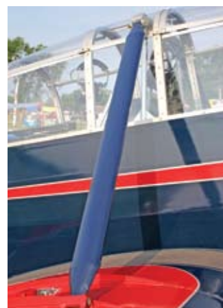
Closeup view of the inboard strut.
