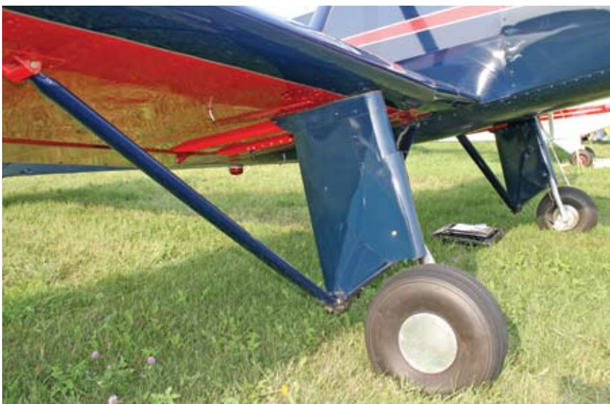
Cleveland brakes have replaced the original Goodyear brakes.
