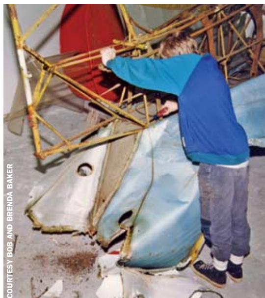
Mark Baker discovered a lot of rust as he helped remove the fabric from the aft longerons.
