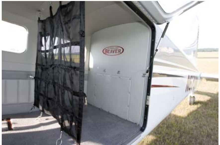
You can carry plenty in a working machine such as this bushplane. A smart-looking Beaver logo is embroidered on the aft bulkhead, with a beefy cargo net installed to keep the baggage where it belongs.
