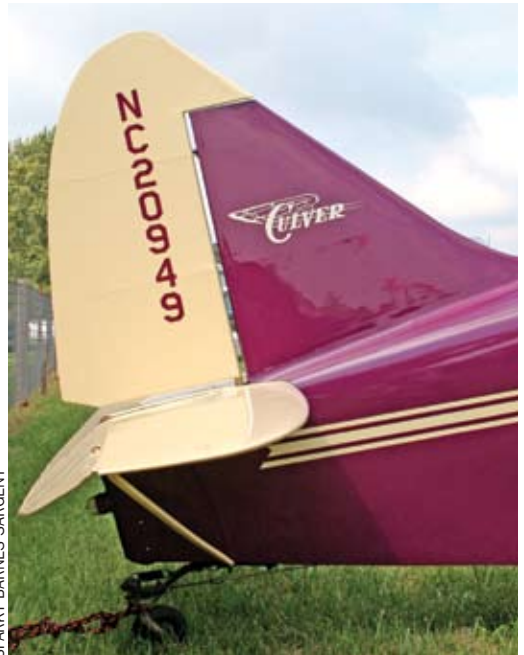
The tail features a fabric gap seal between the horizontal stabilizer and elevator.
