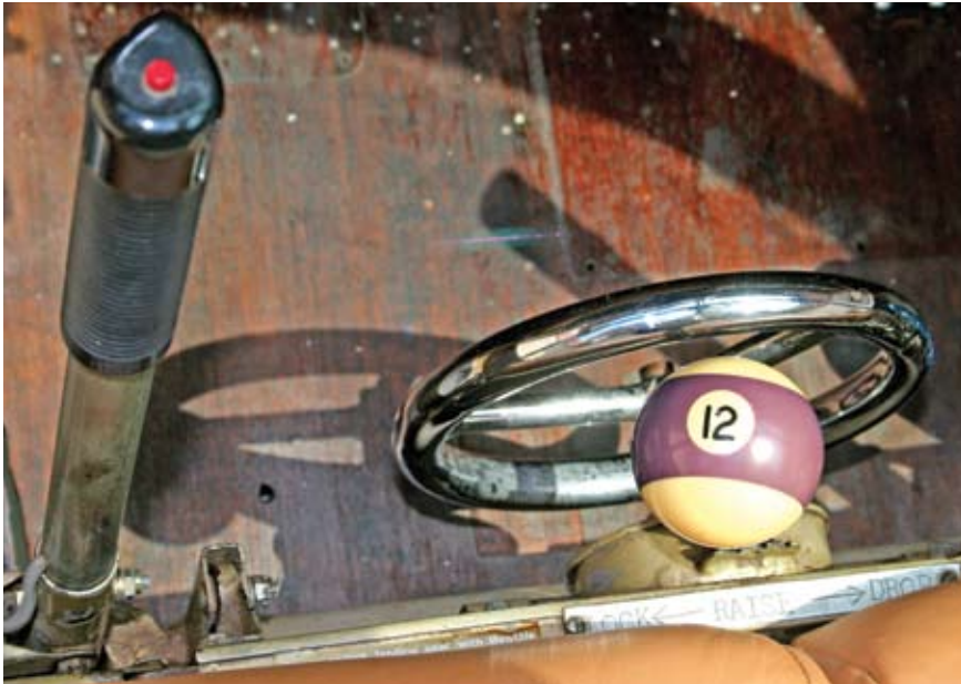
Close-up view of the control stick (left), the pool-ball handle atop the gear lock lever, and chrome wheel, which are used to manually retract and lower the landing gear.
