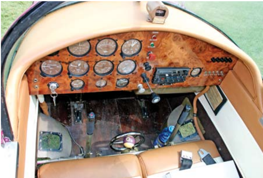
The Model LCA's cockpit. Note the clear windows in the floor panel for viewing the gear position.
