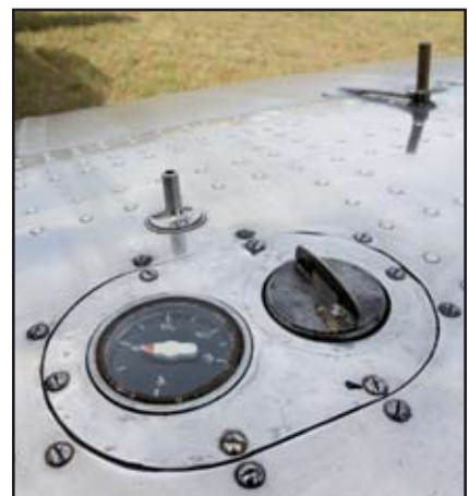
The wing fuel tanks feature the filler neck and mechanical fuel gauge all in one unit.
