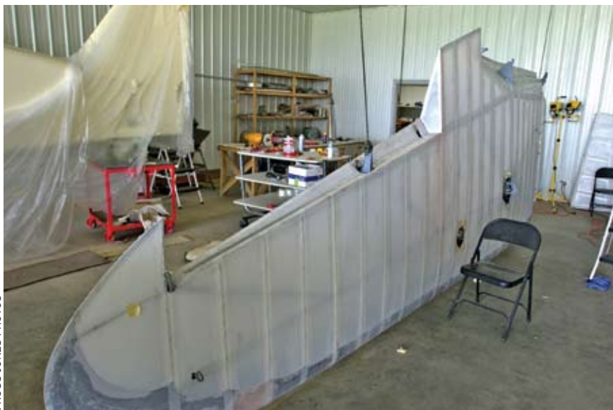
Rib-stitching the Stinson's gullwings was a time-consuming job.
