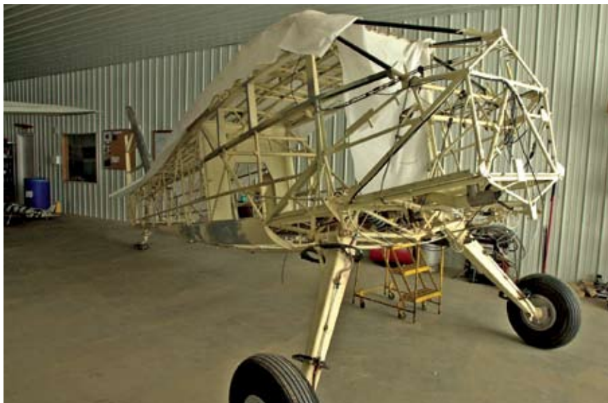
Work on the fuselage is nearing the point of fabric installation.
