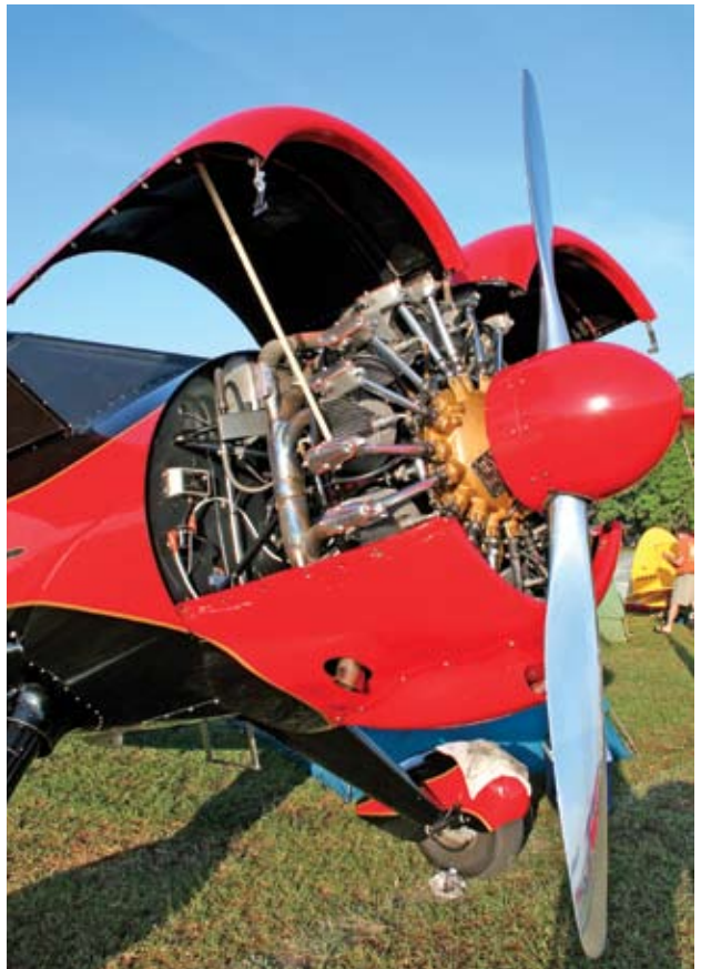
N9116H boasts a 300-hp Lycoming R-680 from Radial Engines Ltd. Note the gullwing style cowling, which provides easy access to the engine and reveals the Stinson's military heritage.
