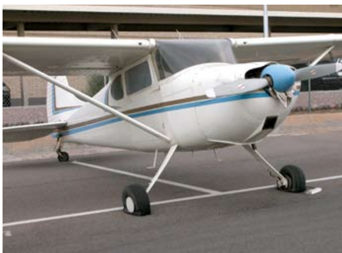
Re-engined with a 160 Lycoming and constant speed prop, this promising looking C-170 is a project, not a ready-to-go used airplane if for no other reason than it hasn't flown for well over a decade. Even though the desert has preserved its metal, the engine is toast. Ditto many of the instruments. If the price is right, this is a clean airframe to work with. The tires might need some attention.
