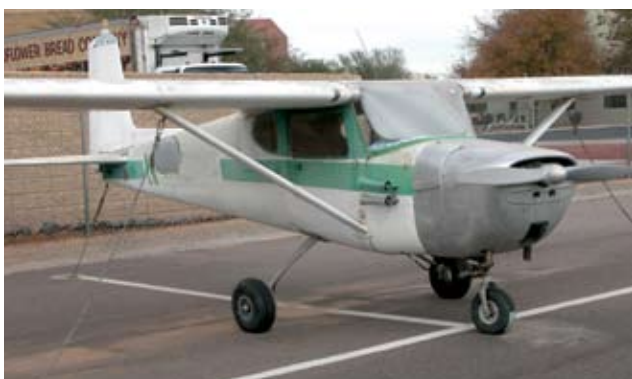
This is a very early, first year production C-150 and the plastic interior is amazingly complete and undamaged. A quick walk around says it also has straight sheet metal, not surprising, considering it hasn't flown since around 1980. Even though the current owner put new tires on it and poured gas into it to get it running, the engine is still probably full of trash, most of it busy eating bearings. Also, the inside of the wings shows some corrosion powder on the top skins. What else is there we can't see? A Long Beach, CA sticker under the tail explains the skin corrosion. Just because you find an airplane in Arizona, doesn't mean it's lived there all its life.
