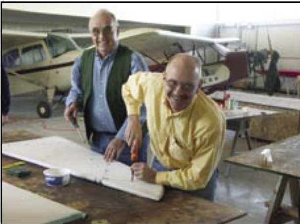
Marty Gallagher and Jim Franseen are having entirely too much fun as they secure the inner fabric tapes to the structure of the elevator using PK screws and small washers.
