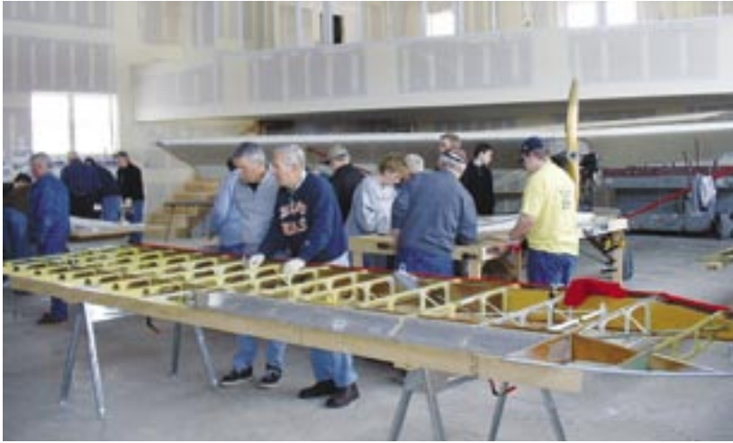
All primed and inspected, the wings are laid out on a pair of sawhorses with long boards running spanwise to evenly support the wings while they are covered. Frank Herdzina's hangar at Poplar Grove was the site donated for the Chapter 1414 Covering Workshop.
