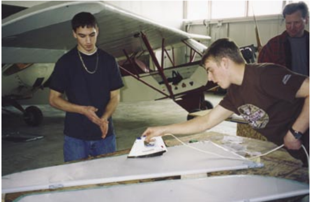
Carl Geiger looks over as Chris Fisher and Rob Fry heat shrink the covering on the horizontal stabilizer of the Champ.
