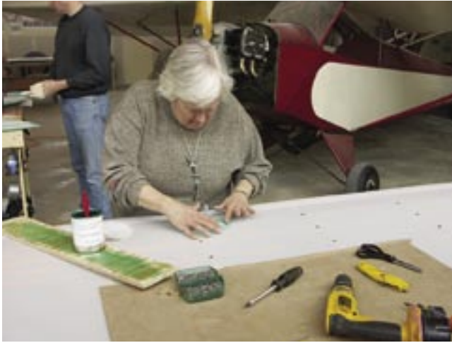
Carol L. Von Bosse concentrates as she glues a reinforcement patch in place over an inspection ring. You can see the PK screws and washers used on the post-war Aeroncas, in lieu of ribstitching.
